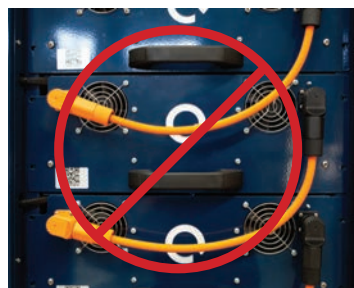
INCORRECT Cable is covering fan
