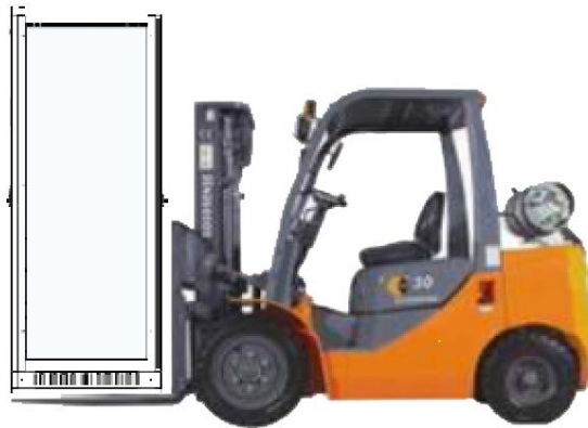
Fig. 4-1 Moving STS Cabinet
